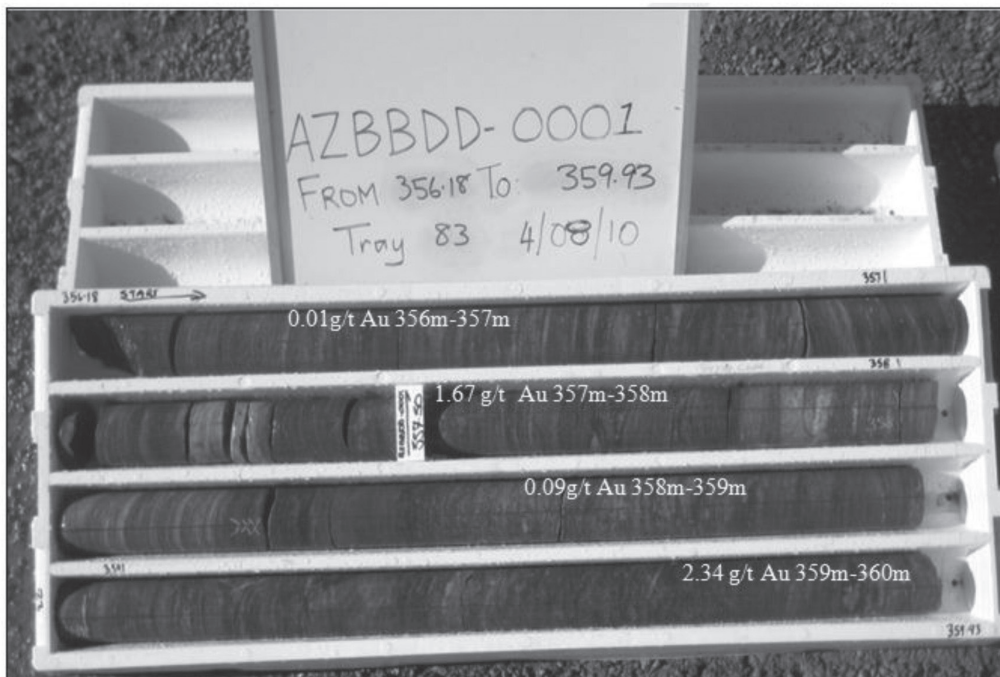
Figure 11. AZBBDD-0001 an example of mineralisation from 354.42m-360.0m which resulted in 5.58m @ 1.93g/t Au. This hole was drilled under the Bacchus pit.
