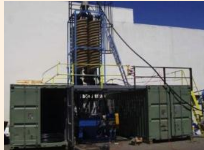
50tph mobile spiral plant (example)
