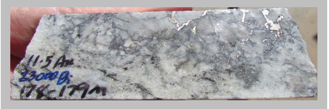
An example of the high-grade gold bismuth mineralisation in the core of the Elaine copper cobalt REE Thorium deposit. Intercept is 11.5g/t gold, 2.3% bismuth, 0.28% copper from 178 to 179m.
