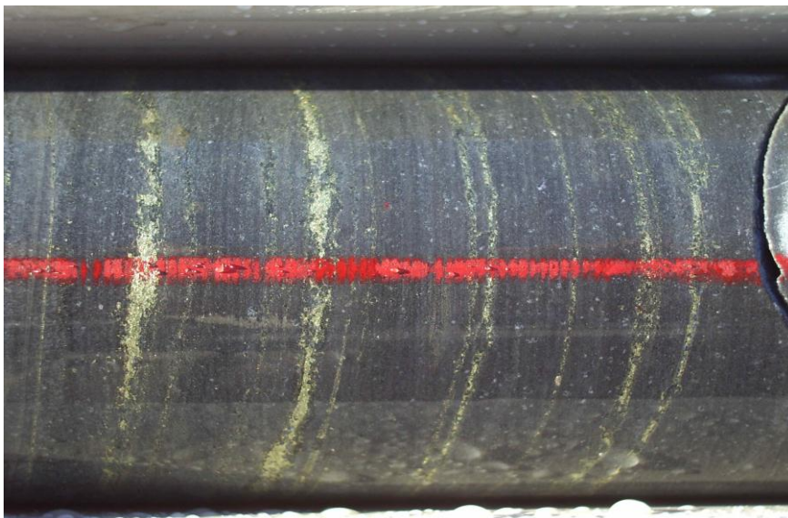
Typical copper sulphide mineralisation from 342.6 metres depth in KKDD 401 (represented by the yellowish-brassy coloured chalcopyrite). In this case the finely laminated chalcopyrite is replacing very thin carbonate-rich beds in the original siltstones of the prospective sequence.
