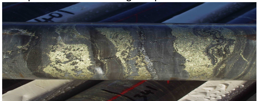
Copper/iron sulphide mineralisation in drill core from KKDD401
