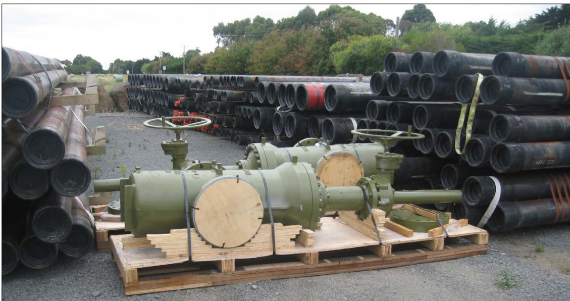
Figure 4: Well casings and wellhead valves in storage at Koroit ready for commencing the drilling and testing of two deep wells in the Stage 1 Koroit geothermal program
