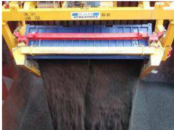
Figure 10: Rotating Spreader in operation
