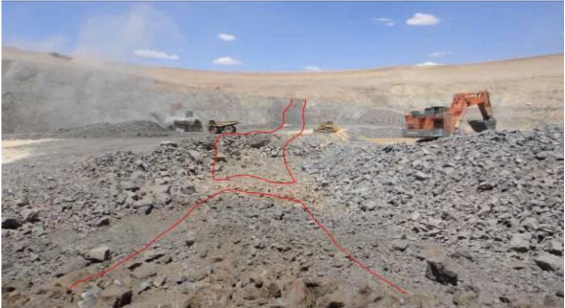
Starter Pit Looking East Showing 95RL floor at the east end (Photo taken 01/01/2012) Red Outline Delineating Ore Zone
