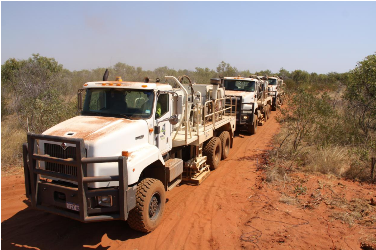
EP 438 Canning Basin - Recording the Athos Multifold 2D Seismic Survey with Terrex Seismic in September 2011. Geophones are located on the right hand side of the photo.
