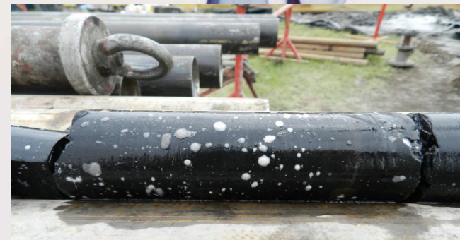
KA02 311 m- Sample of Coal with Gassy bubble desorption
