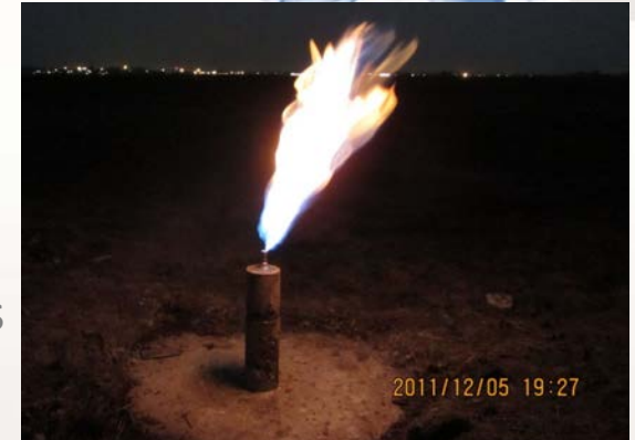
KA06 360m - controlled flaring of spontaneous gas flow
