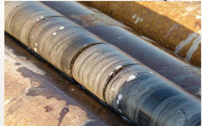
KA04 – Sample of Carbonaceous Mudstones with Gassy bubbles desorption
