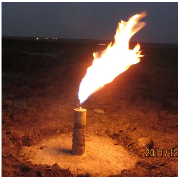
Figure 1: Flaring of spontaneous gas flow from KA-06 (since December 2011)
