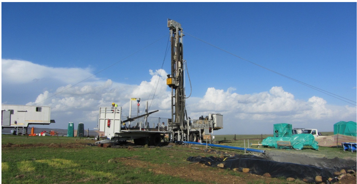
Photograph 1: Gas Production rig spudding well KA-03PT, Amersfoort Project, Mpumalanga, South Africa
