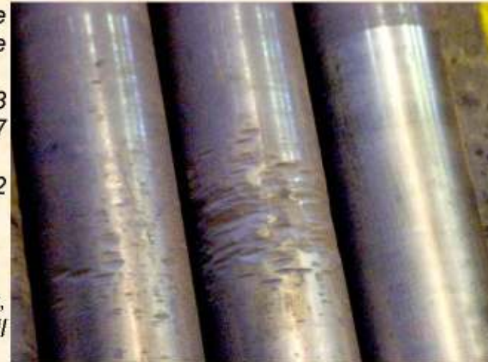
Two hardened steel rolls on left compared with Laser-Bond™ roll on right after same service.
