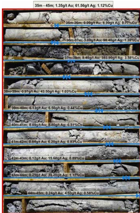
BMS-007a, 35 to 45 metre interval averaging 1.35g/t gold, 61.56g/t silver and 1.12% copper.
