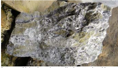
Layong Vein breccia mullock sample. Note stockwork and vuggy silica infill on breccia with galena (lead) and pyrite mineralisation. Typical intermediate sulphidation assemblage and textures.
