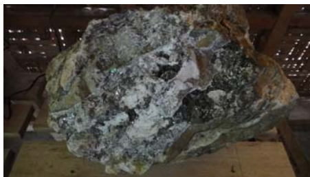
Layong Vein breccia mullock sample. Note stockwork and vuggy silica infill on breccia with galena (lead) and sphalerite (zinc) mineralisation. Typical intermediate sulphidation assemblage and textures.
