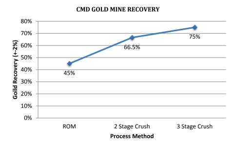
An evaluation of the preferred processing method is ongoing however as shown in Figure 2 below, there appears to be advantages in 2 Stage Crushing only as this provides a similar margin to 3 Stage Crushing, but at lower costs. The CMD Gold Mine process plant also has excess capacity in the primary and secondary crushing circuits, which would enable a higher throughput than achievable through the tertiary crushing circuit.
