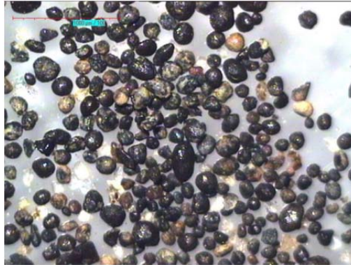
Microscopic pictures of Concentrate (binocular 100 x magnification)
