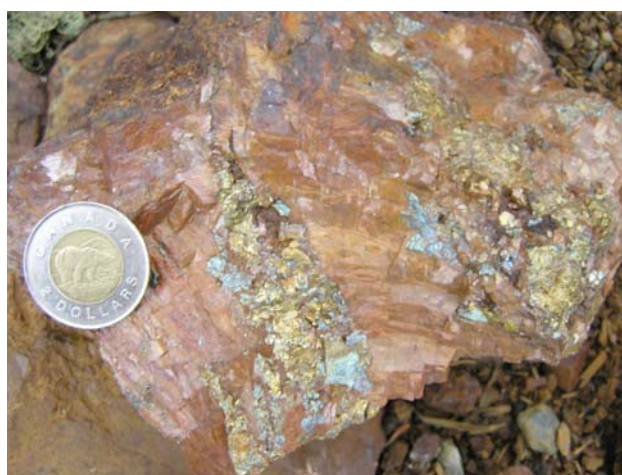
Figure 2: Iron carbonate-chalcopyrite breccia from the Copper Lake historic workings. This sample assayed 2.7% copper and 1.13 g/t gold.
