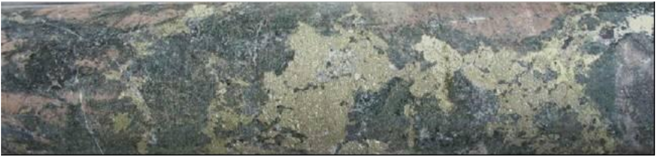
Figure 12 – IOCG style alteration and mineralisation in the Boomara Project (KDD13, 375.6m)
