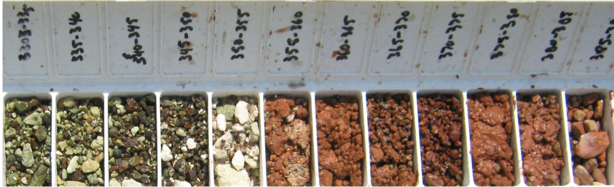
Figure 3(a): Weakly magnetic and intense epidote (green) altered and hornfelsed (dark brown) rhyolite tuff to 350ft (106m) along western contact with bleached and haematite (brown) dusted fine grained intrusive rhyolite in AW12-08.
