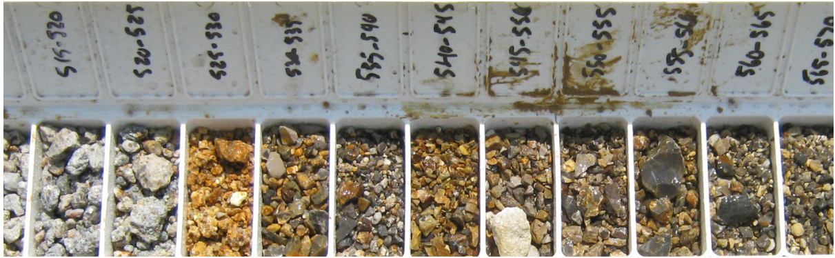
Figure 3(b): Silica flooded and weakly brecciated eastern contact with rhyolite intrusive pipe at 530 ft (161m) in AW12-08. 520-540ft returned anomalous Ag (2.71ppm); As (271ppm); Sb (17.5ppm) and 525-535ft returned 0.17g/t Au.
