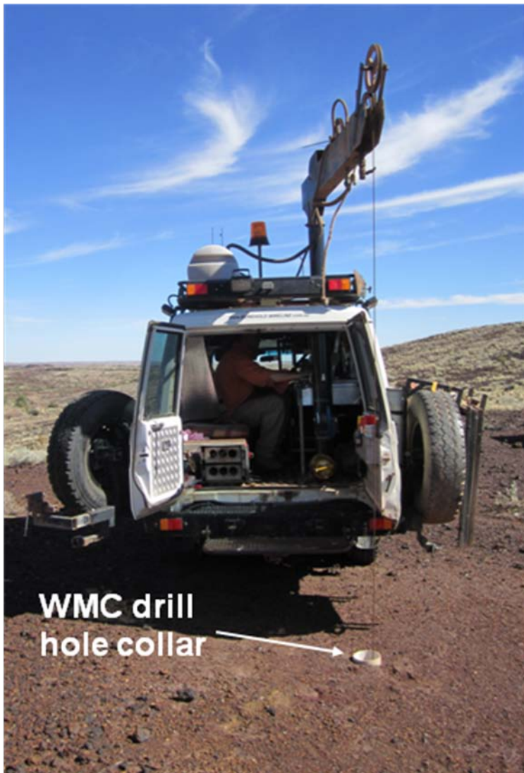
Figure 6: Downhole logging completed during December 2011 at Western Spur.
