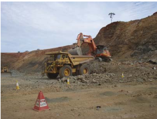
1 st bucket of high grade ore going into Cat777B dump truck.
