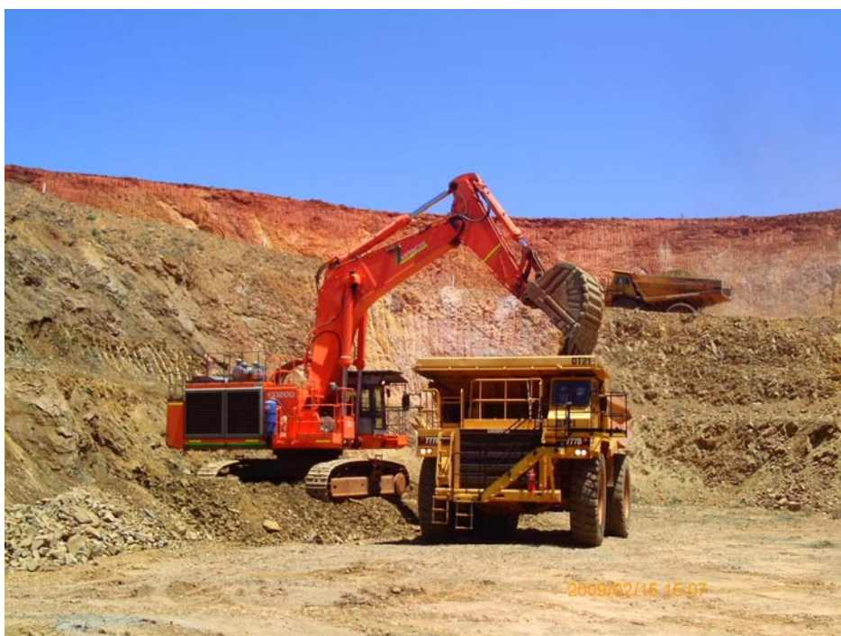
Figure 5. Mining activity in the pit is well advanced. Nex has a fleet 777B Caterpillar Trucks on site.
