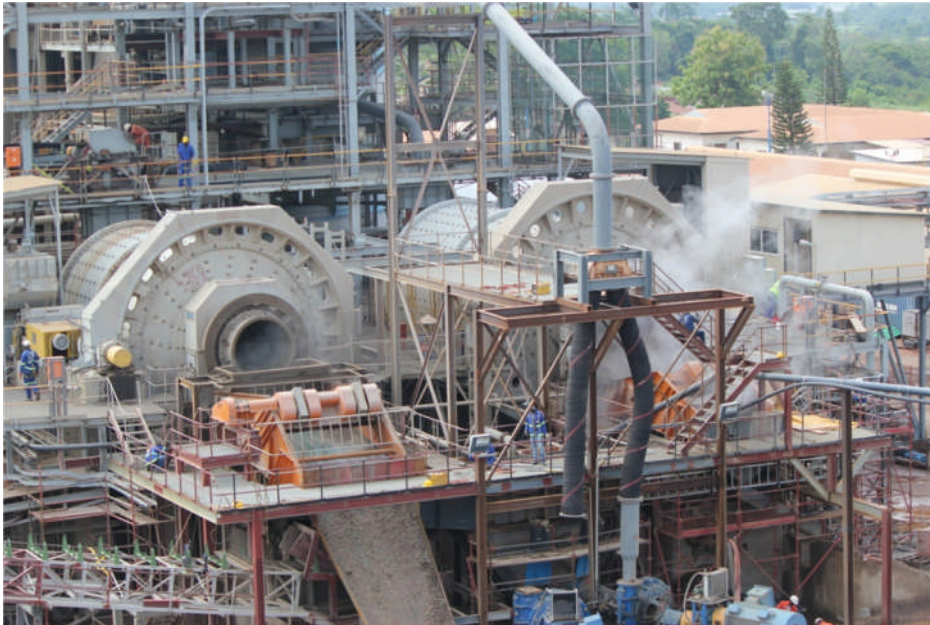
Both SAG and Ball mills operational (SAG mill to the left and Ball mill to the right)
