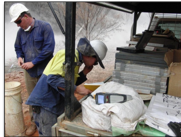
Field XRF being used during 2011 Arganara drill program
