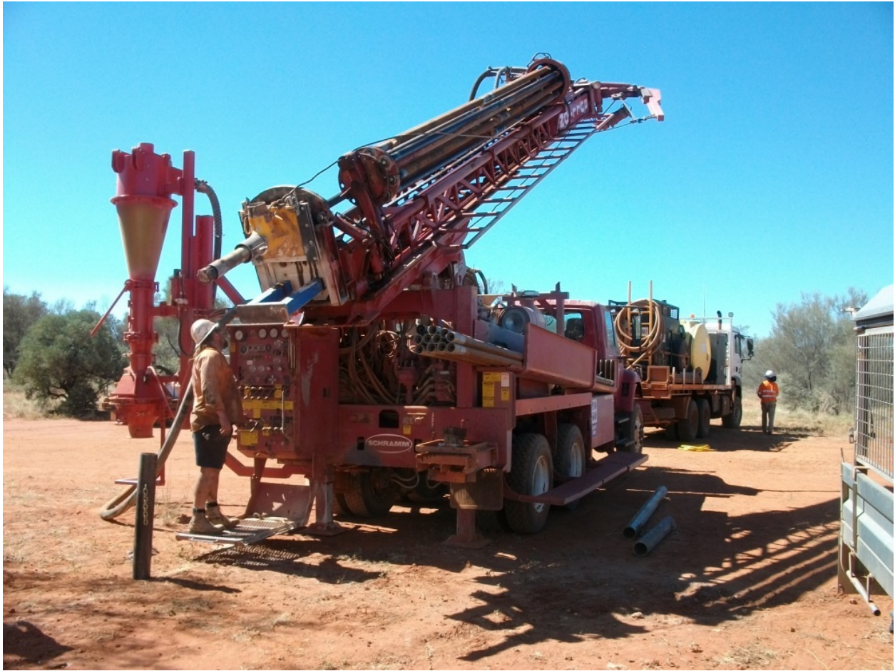
Bullion Drilling Setting up Rig for first RC hole, Arganara Phase 3 Program – May 2012
