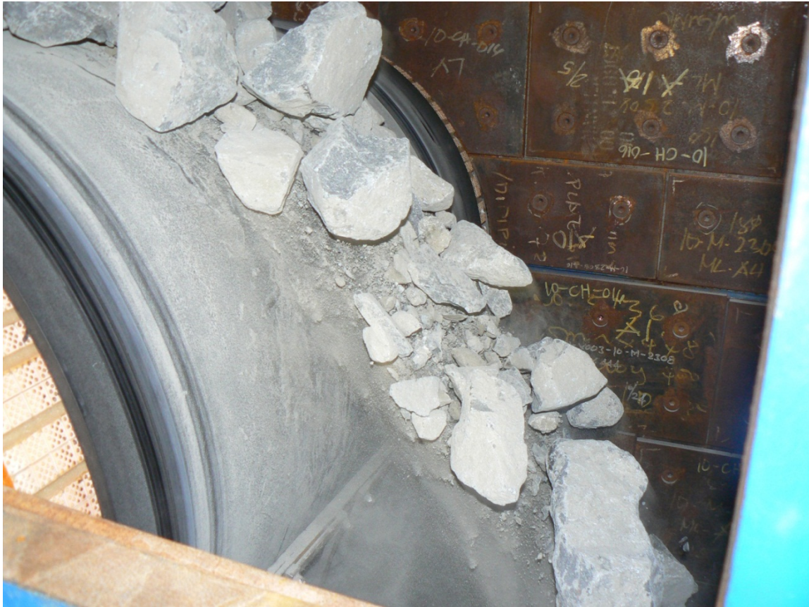
Figure 2 – Commissioning the SAG Mill on rock
