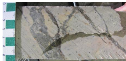
Wongoni Project Drillhole DD92HV14 - 146m Pyrite veining in silica- sericite(phengite)-kaolinite- pyrite altered volcaniclastic
