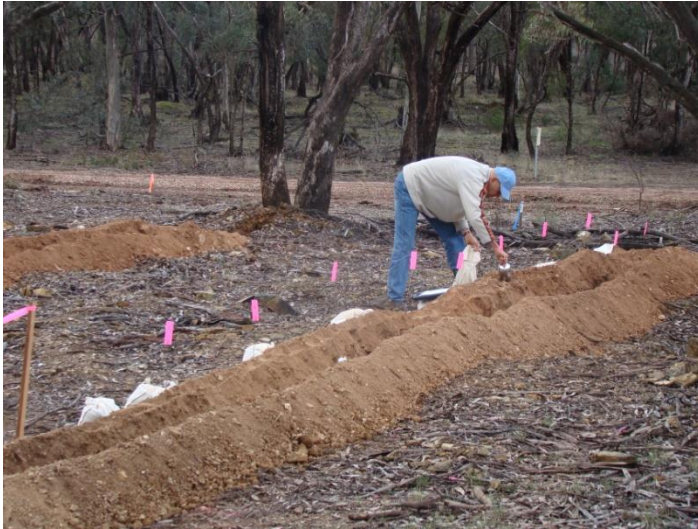
Surface trenching and grade control sampling
