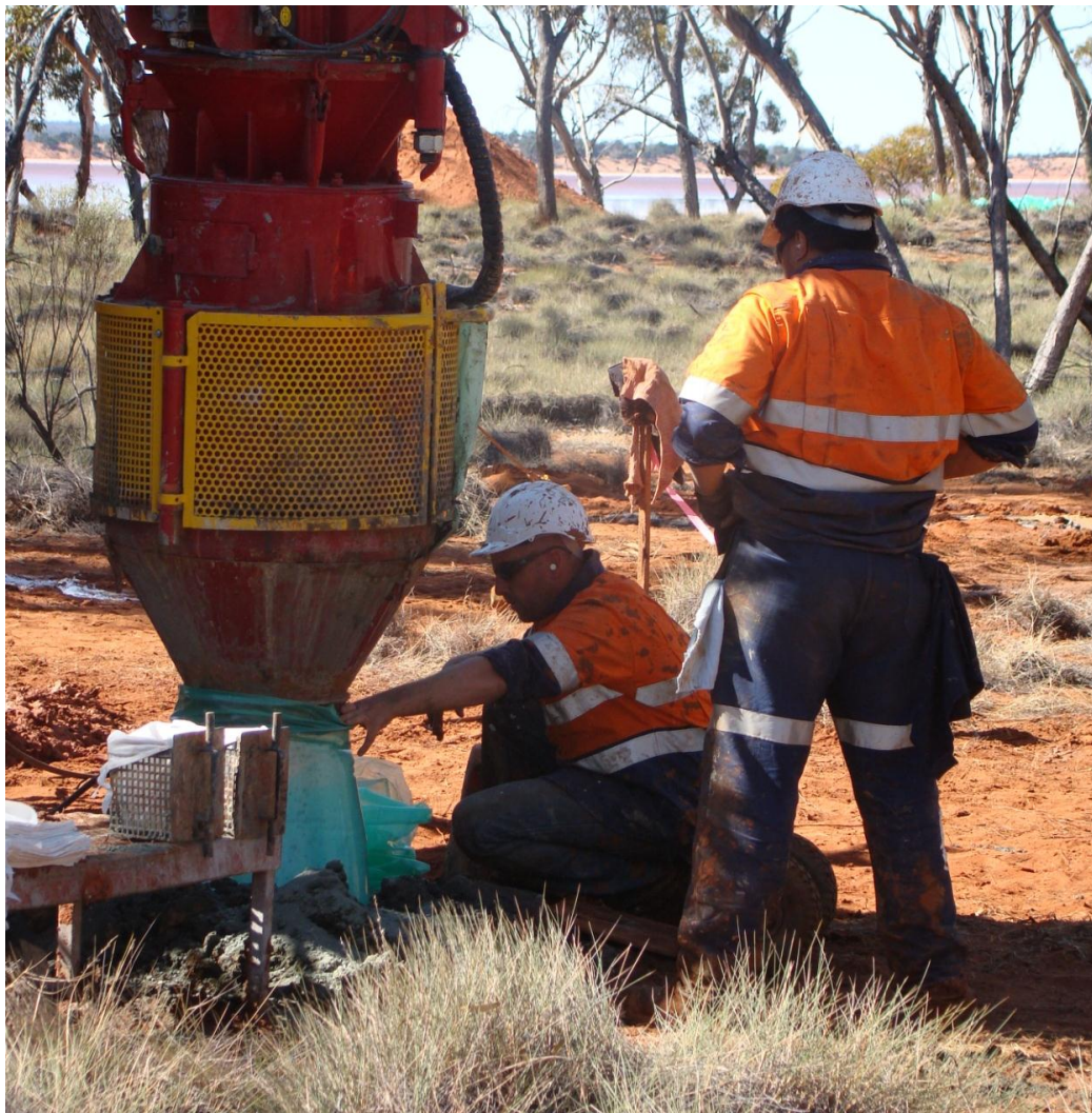
RC Drilling at the Burns Prospect
