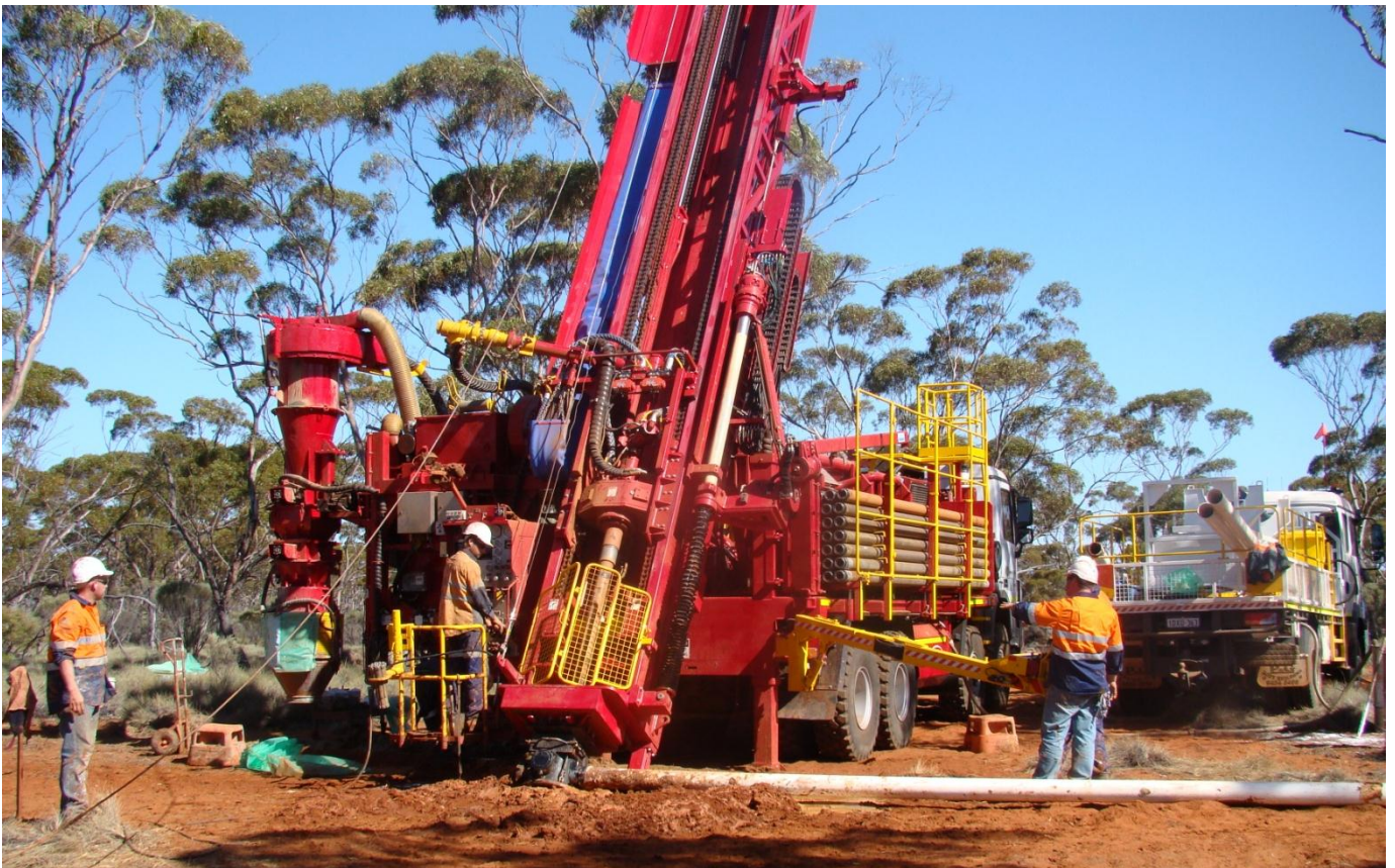
RC Drilling at the Burns Prospect
