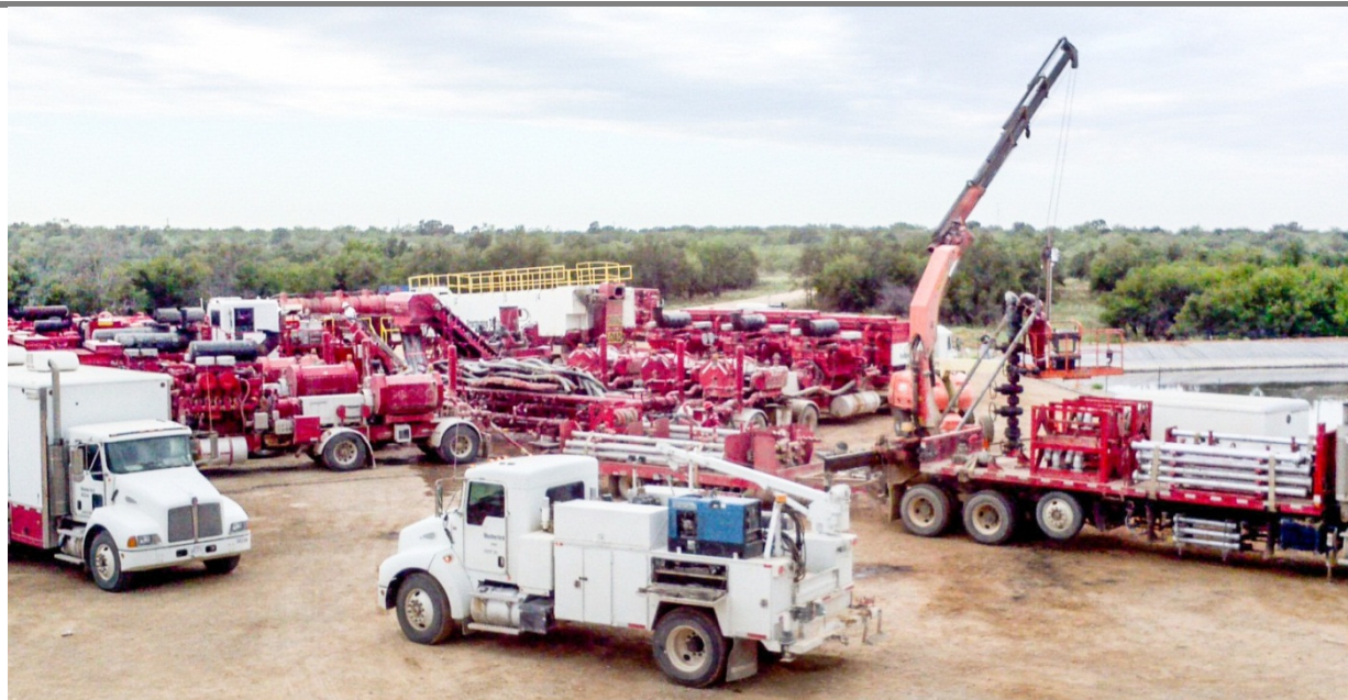
Comanche Test Well # 1 undergoing fracture stimulation
