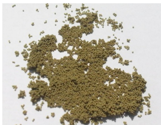
Figure 1 – Dow Chemical selective nickel low-pH Ion Exchange Resin
