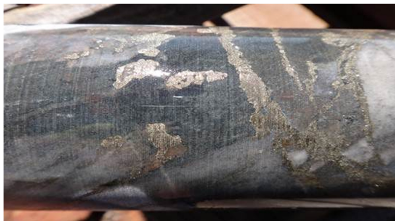
Figure 5 –Pyrite and chalcopyrite in stringers and on joint planes in black shale rock at 415.4m
