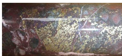
Depth 256.6 metres: Chalcopyrite-pyrite in microdiorite endoskarn. From interval 2m @ 1.40% Cu.
