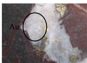
Depth 254.5 metres: Native Au-chalcopyrite-pyrite in skarn. From interval 2m @ 15.4 g/t Au.
