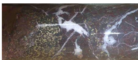
Depth 262.2 metres: Chalcopyrite-pyrite in microdiorite endoskarn. From interval 1m @ 2.25% Cu.
