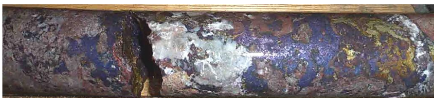
Depth 235.3 metres: Chalcopyrite-pyrite-covellite in skarn. From interval 10m @ 0.97% Cu.
