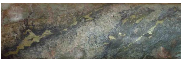
Depth 229.5 metres: Chalcopyrite-pyrite-covellite in skarn. From interval 10m @ 0.97% Cu.
