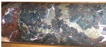
Depth 259.7 metres: Chalcopyrite-pyrite in microdiorite endoskarn. From interval 2m @ 1.40% Cu.
