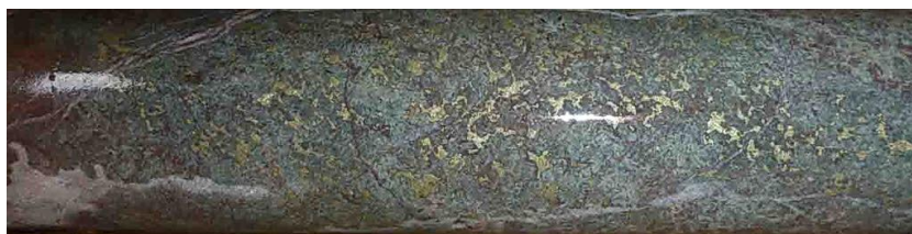
Depth 263.7 metres: Chalcopyrite-pyrite in microdiorite endoskarn. From interval 1m @ 2.05% Cu.
