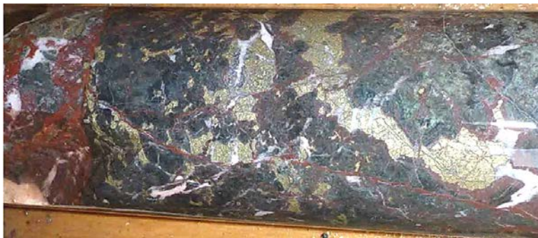
Depth 259.7 metres: Chalcopryite-pyrite in microdiorite endoskarn. From interval 2m @ 1.40% Cu.
