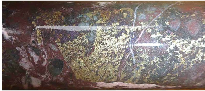
Depth 256.6 metres: Chalcopryite-pyrite in microdiorite endoskarn. From interval 2m @ 1.40% Cu.
