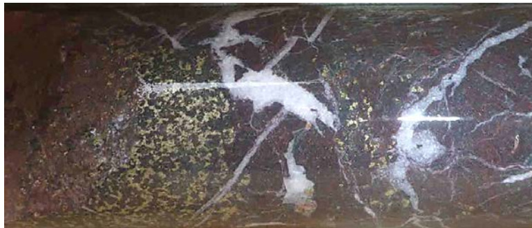
Depth 262.2 metres: Chalcopryite-pyrite in microdiorite endoskarn. From interval 1m @ 2.25% Cu.
