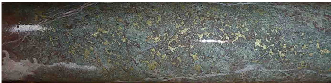
Depth 263.7 metres: Chalcopryite-pyrite in microdiorite endoskarn. From interval 1m @ 2.05% Cu.
