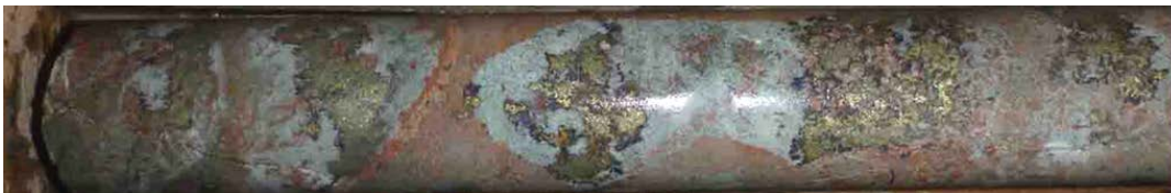
Depth 230 metres: Chalcopyrite-pyrite-covellite in skarn. From interval 10m @ 0.97% Cu.
