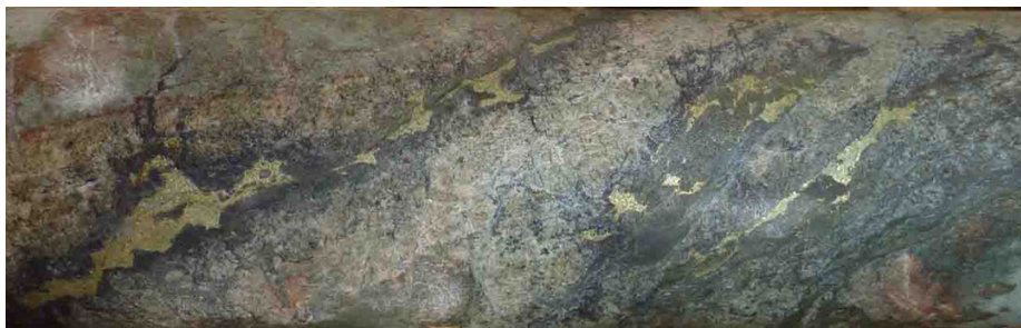
Depth 229.5 metres: Chalcopyrite-pyrite-covellite in skarn. From interval 10m @ 0.97% Cu.
