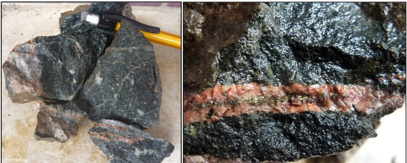
Figure 2: (Left) Example of fine chalcopyrite filled millimetre wide veinlets in microdiorite-diorite and (right) feldspar vein with centreline filled with chalcopyrite-pyrite.
