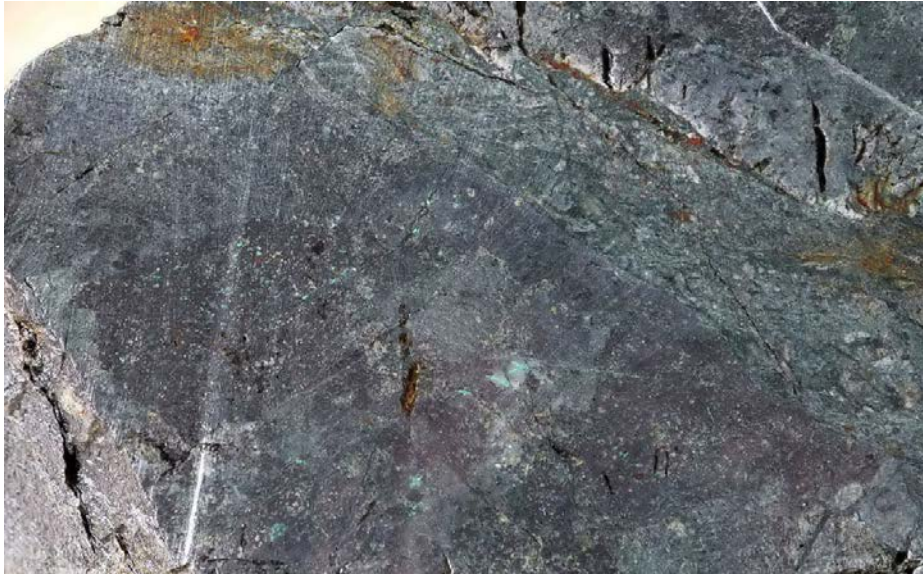
Figure 3: (Left) Example of fine green disseminated malachite after chalcopyrite in weathered sheared and altered microdiorite. Similar material probably gives rise to the widespread elevated copper background anomalism.
