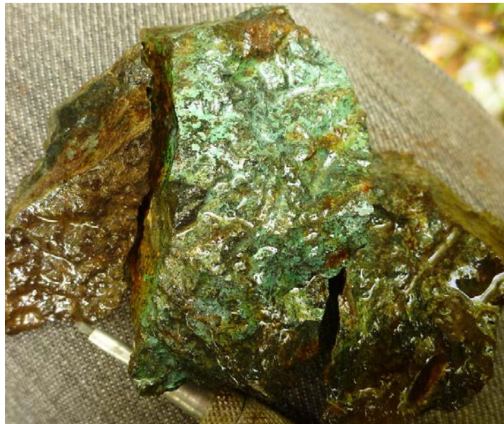
Figure 2: Malachite staining on microdiorite derived from magnetite \pm sulphide \pm silica veinlet fracture fill.
