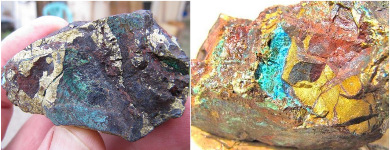
Figure 2: Massive sulphide segregation from composite channel outcrop of chalcopyrite and bornite(?) rich endoskarn.
