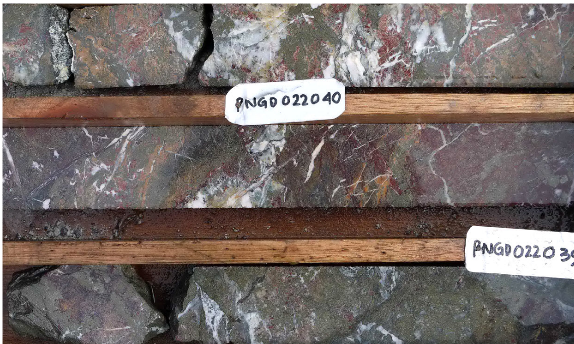
Figure 14: High grade Au interval at 73-75 metres in sulphide-rich endoskarn (Sample PNGD022039 = 58g/t Au).
