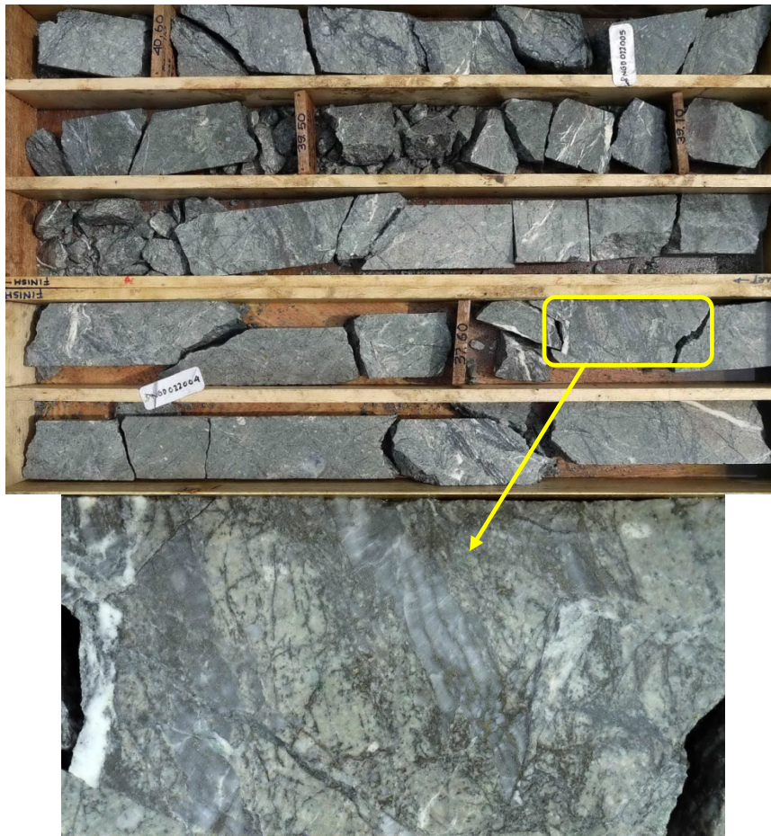
Figure 7: Higher temperature stock work and crystalline quartz veins in microdiorite 36-40 metres down hole. Detail of deformed laminated quartz veins with sulphide centreline and fracture fill and alteration in quartz diorite.
