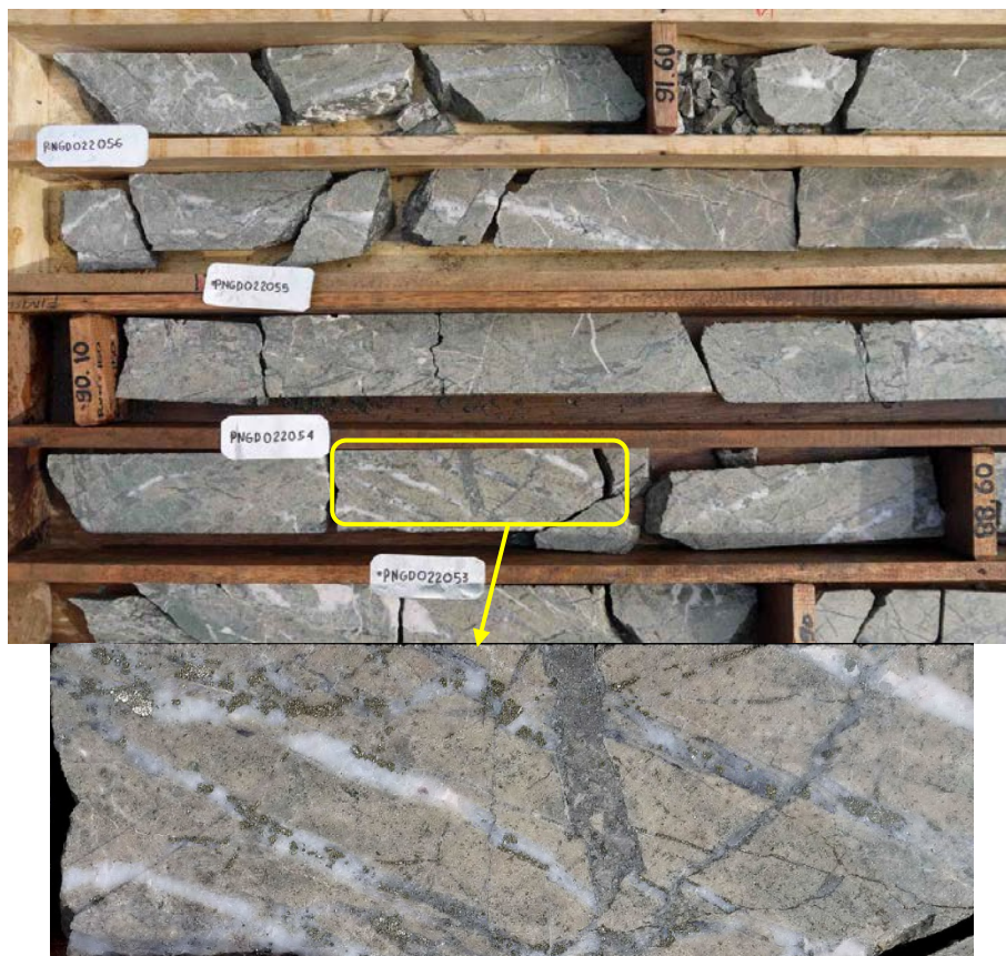
Figure 15: Examples of quartz stockwork veinlets 88 to 90 metres down hole. Detail showing multiple vein formation textures and relation to sulphide introduction.
