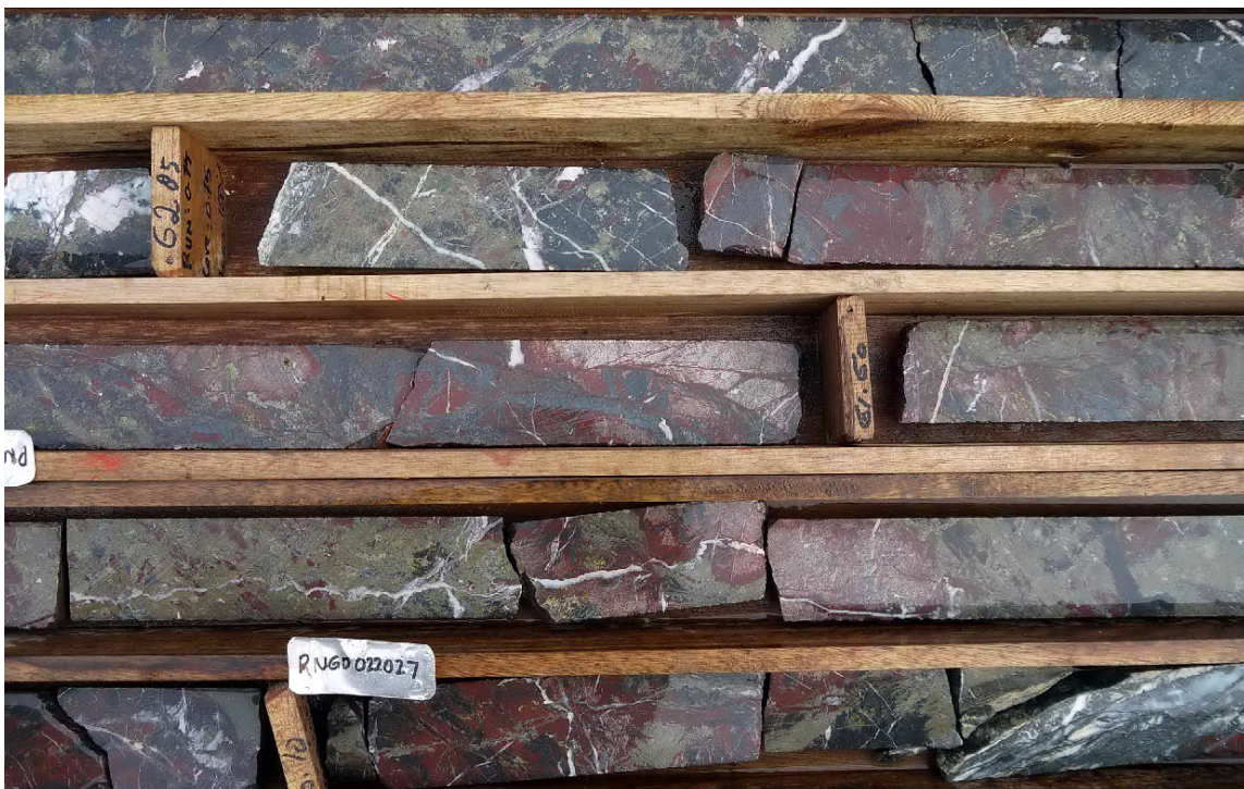
Figure 12: Core interval 60-62 metres showing intersection of replacement endoskarn in microdiorite. Note hydrothermal magnetite growths and extensive sulphide development. This section has elevated Au values. Detailed views are shown below.
