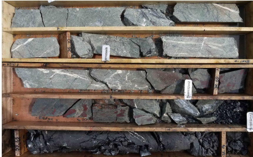
Figure 6: Contact between sediments and microdiorite at 33.65 metres.
