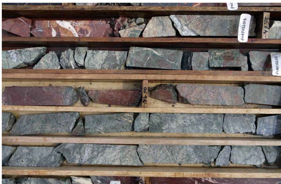
Figure 9: Porphyry-related quartz stockwork veins 44-47 m depth. Detailed photos are shown below.
