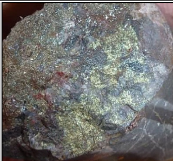
Figure 13: Intersection of sulphide-rich endoskarn in microdiorite in section from 60-65 metres coincident with anomalous Au zone. Note hydrothermal magnetite vein fill in upper photograph.
