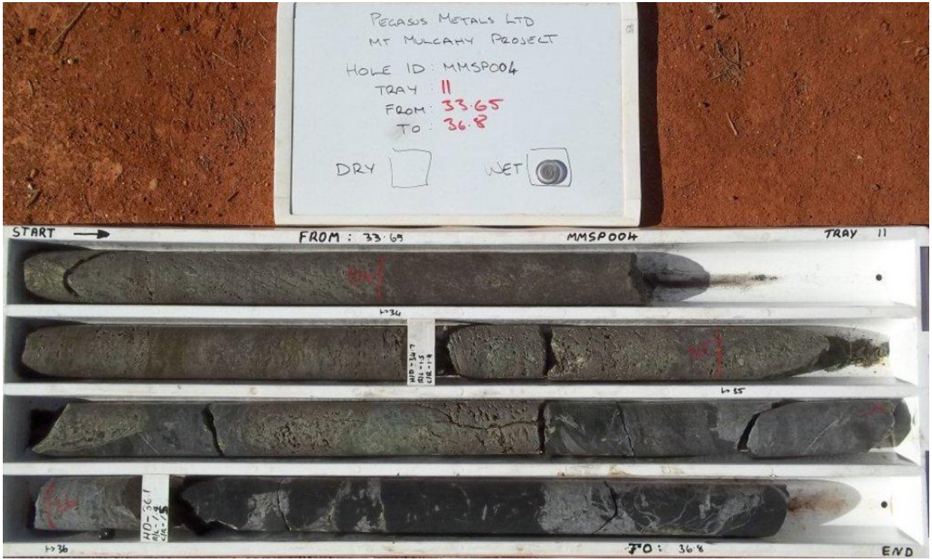
MMSP004 core photo showing lower part of intercept containing massive chalcopyrite/sphalerite mineralisation and lower contact with sediments.
