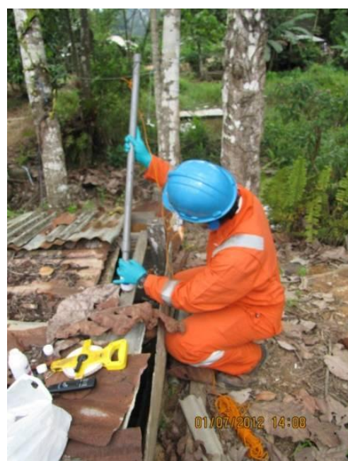
Well water sampling
