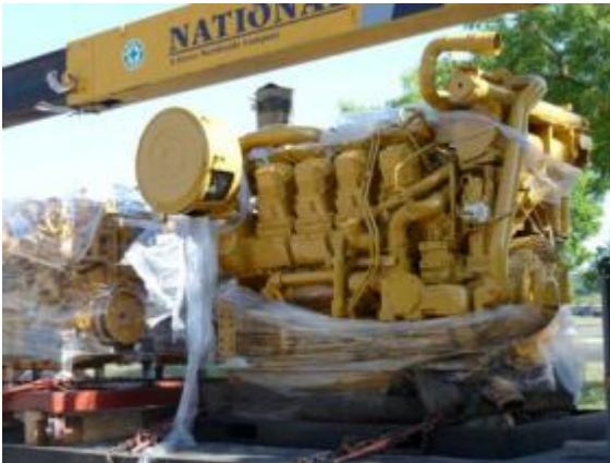
CAT 3500 Diesel Engine being unloaded at Clark
