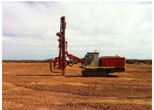
Blast hole drilling at Genesis open pit
