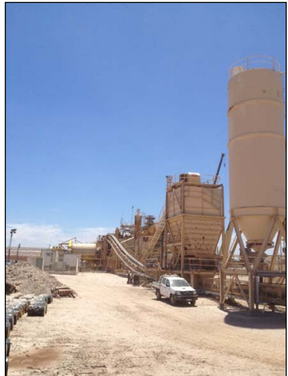
Figure 4: Photo of Lakewood Gold Processing Facility upgraded circuit showing new 150 cubic metre leach tank, materials handling system with 1.6 megawatt ball mill in the background.
