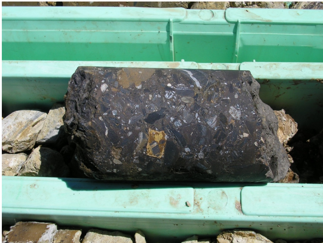
Photo 2 - THD002, 318.5m – Weathered Ironstone Breccia with 1% Cu
