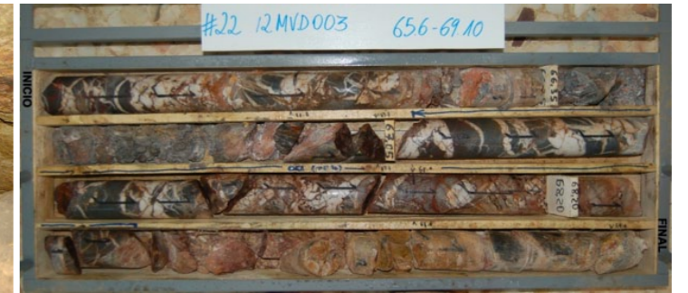
Figure 2c. Veining and brecciation in recently drilled diamond core at Montevejo prospect.
