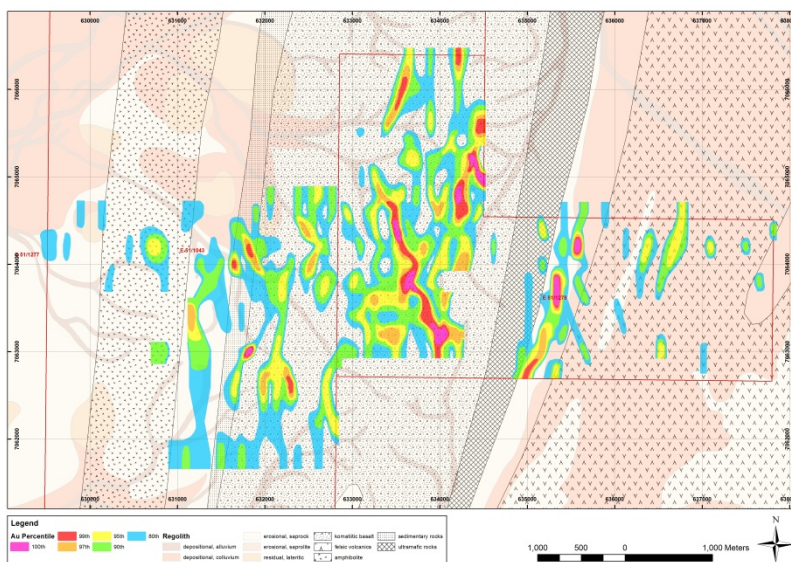
Abbotts South: a 2km long gold in soil anomaly. Sample have been collected on 80m sapling centres and 200m line spacing.
