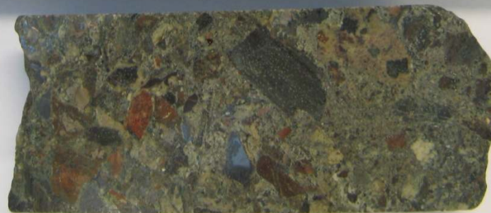
Heterolithic, carbonate breccia (py, cpy, hem)
