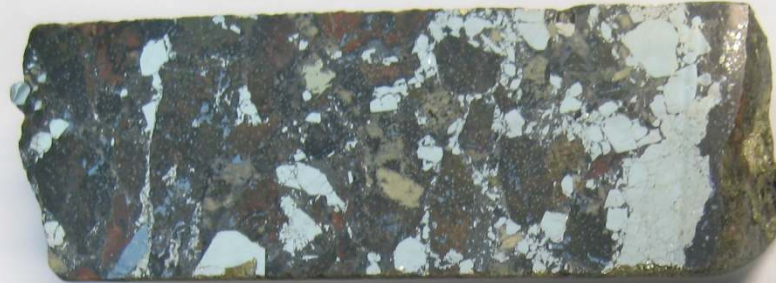
Mineralised, hematite matrix- rich breccia (py, cpy)
