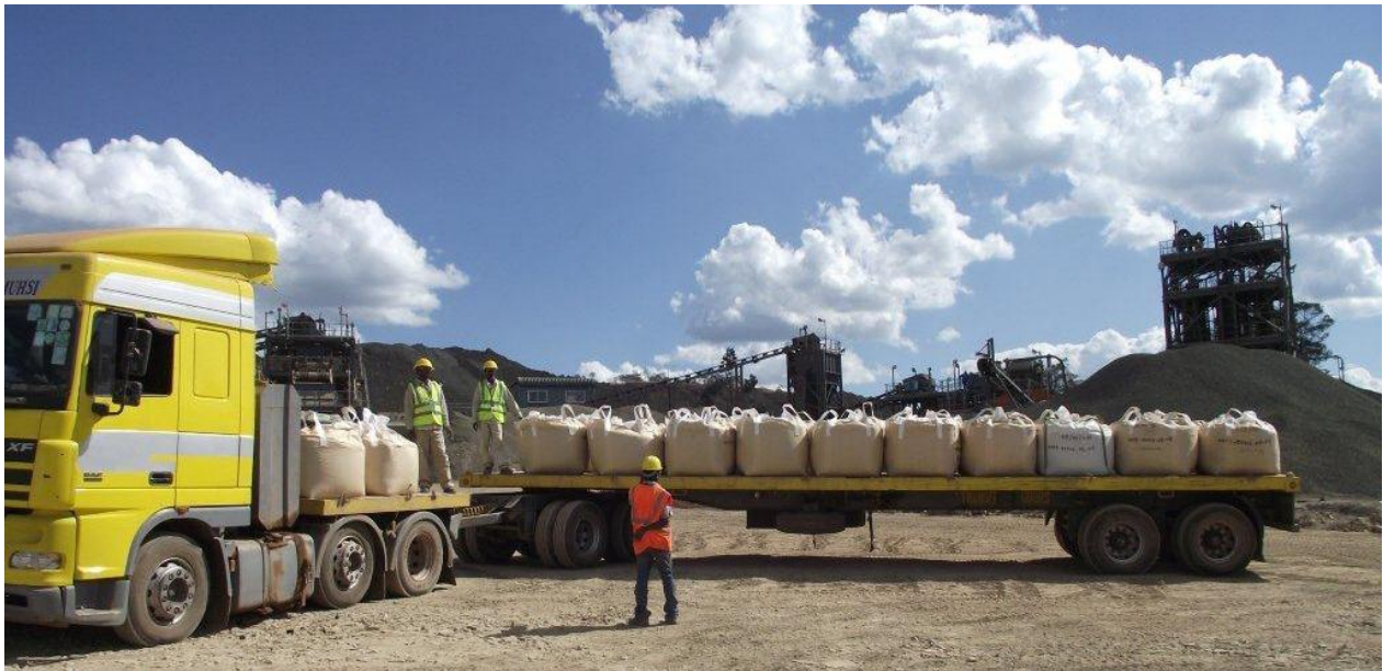
First export load of +25% Cu concentrate leaves Kipoi for Zambia, transported in 1.2t bags
