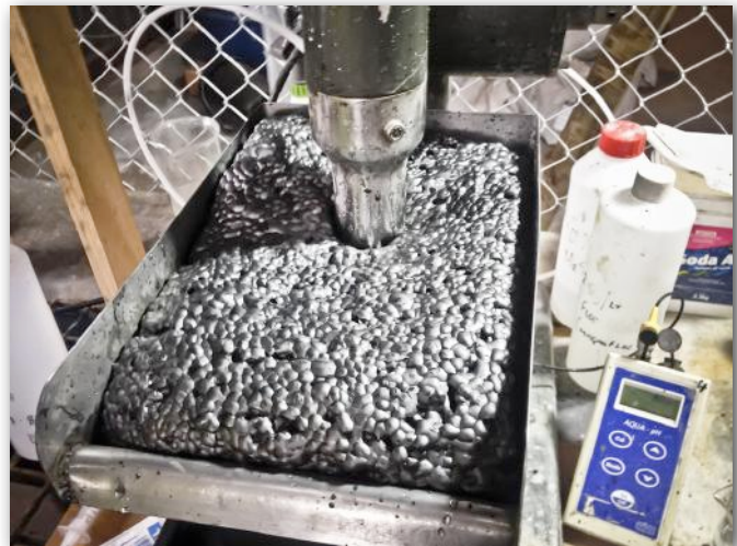
Photo 2. Flotation tests on Nunasvaara graphite underway.
