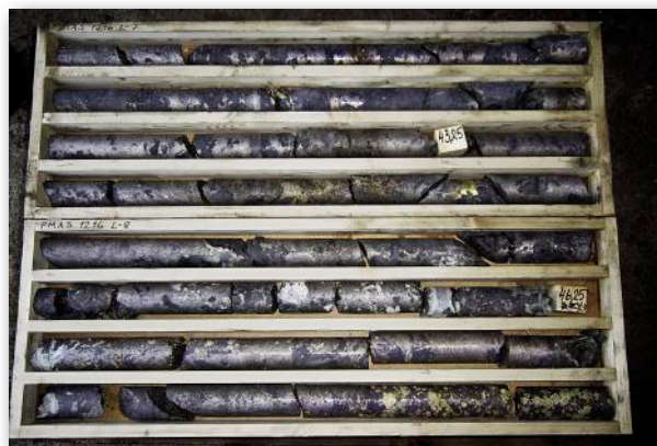
Fig 5. Sulphide zone at 40-47.6m depth, MAS1216 Masugnsbyn.
