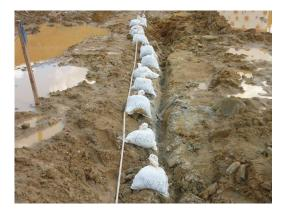
Figure 1. Samples collected along the line of mineralisation in the trial mine pit -6m level
